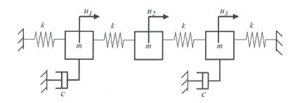
The springs have spring constants k, the masses have mass m, and the damping constants are c. The external forces are given by  $u_1, u_2$ , and  $u_3$ .
